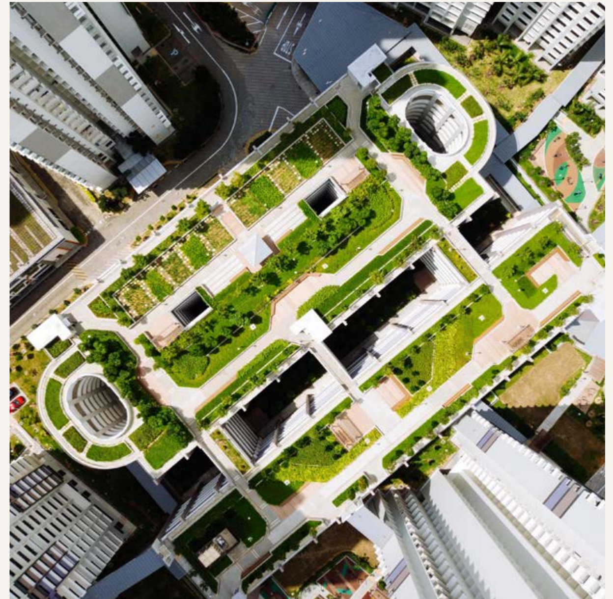
Innovative greening solutions on the rooftops of Housing & Development Board (HDB) flats help to reduce heat emissions from building surfaces and improve the appearance of HDB estates, making the living environment more conducive for residents.
